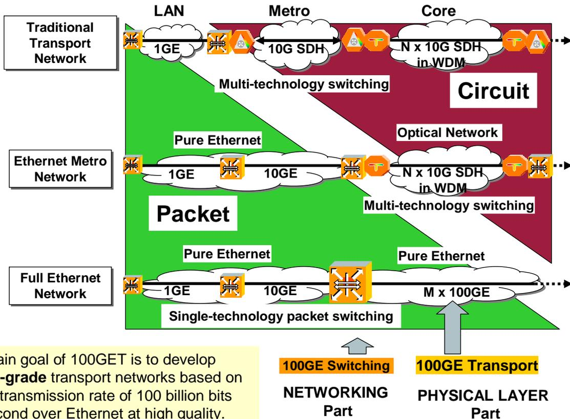
The main goal of 100GET is to develop **carrier-grade** transport networks based on a data transmission rate of 100 billion bits per second over Ethernet at high quality.
